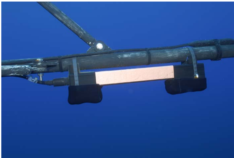
Figure 1. Neoprene caps on each transmissometer for acquiring three dark measurements.
